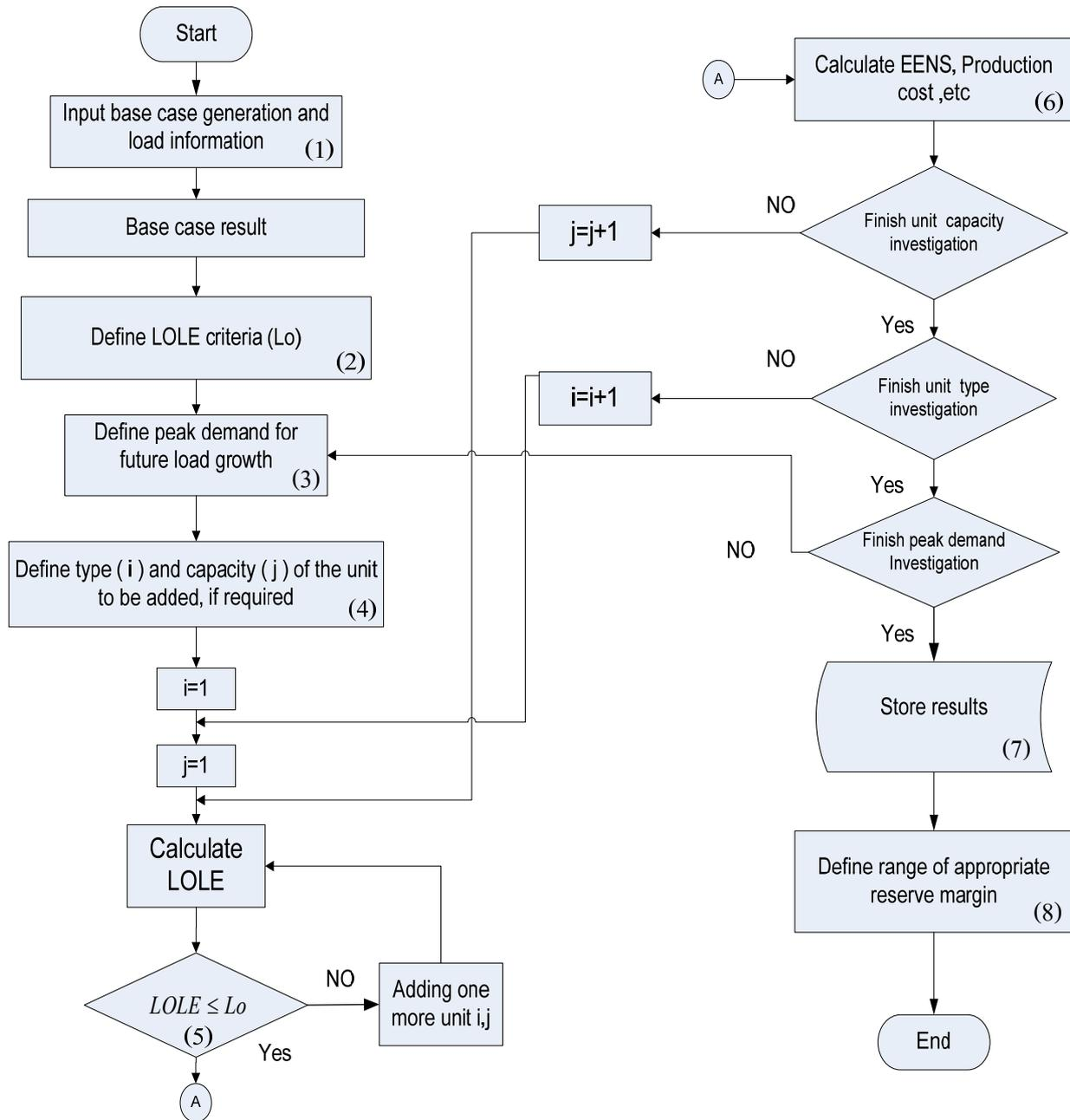
Figure 7 Reserve margin determination based on probabilistic and deterministic methods
