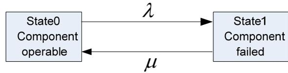
Figure 1 Two-state model for base load unit
