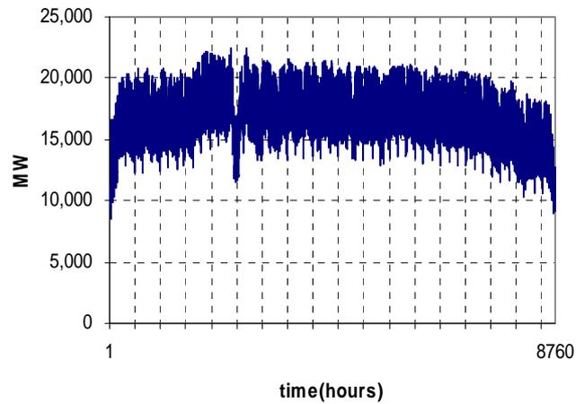
Figure 2 Hourly load curve
