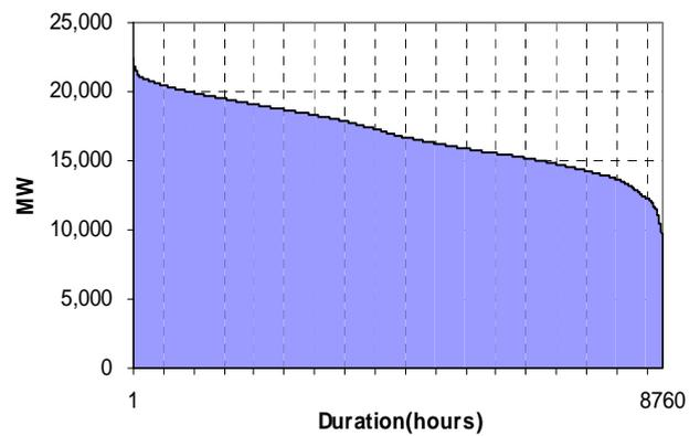
Figure 3 Hourly load duration curve
